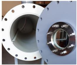
The cheap solution as a pressure chamber or autoclave
